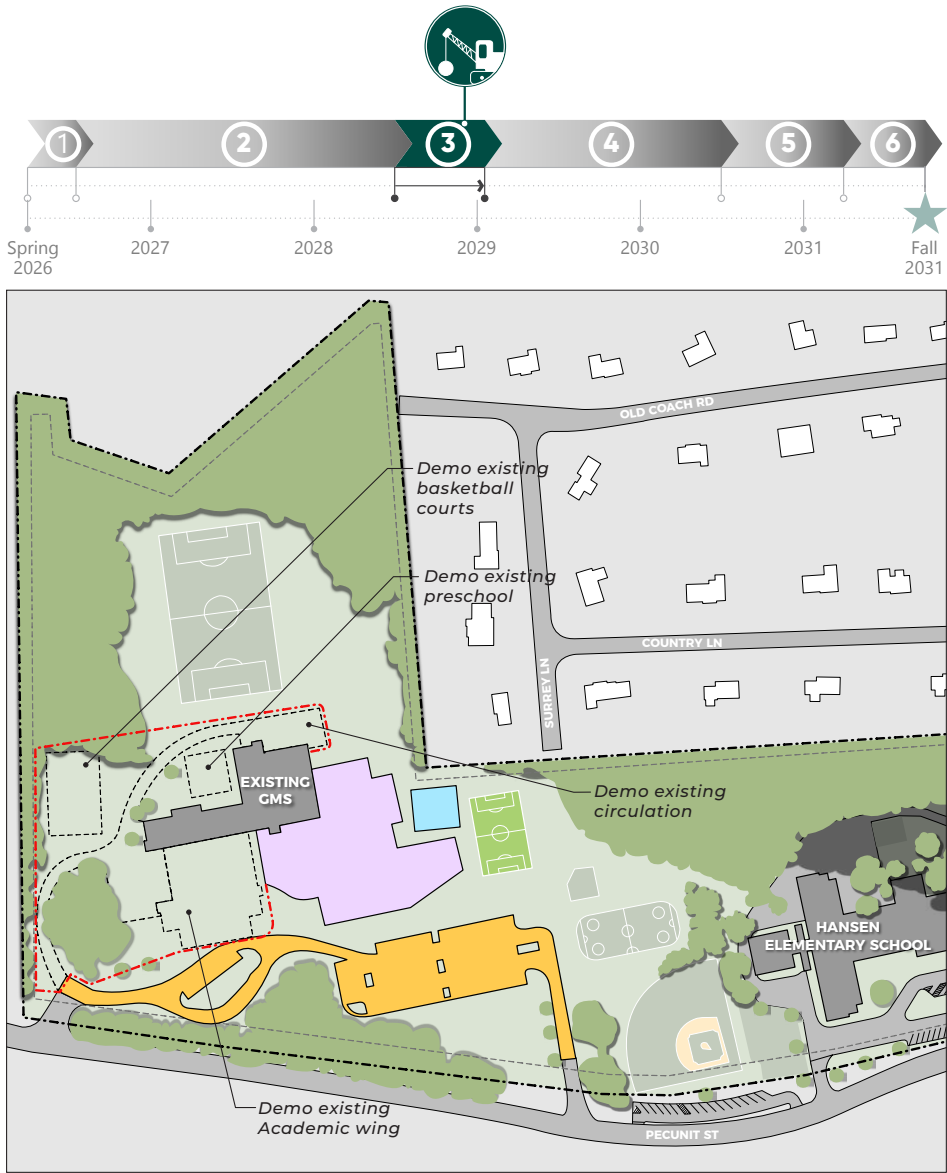
Phase 3 July 2028: Demolition of portion of existing Galvin Middle School academic wing, preschool, outdoor activity space and associated parking & circulation. Temporary shore existing building to remain occupied - cut, cap, and make safe all utilities and install temporary exterior cladding.
